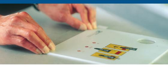
DuraSeal base plates are also suitable for the production of medium and large series. The plates are available with different anodising layer thicknesses, depending on the application. In combination with the highly concentrated PoroPrint silkscreen pastes, you always get an even, durable, colourfast result.
